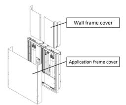
**Included in the package:** BalanceBox® 650, multilanguage manual, wall mounting bracket, steel wall frame cover (power coated) and fasteners, steel application frame cover (powder coated).
